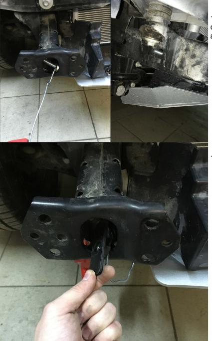
14. Place insert nuts (5) into the chassis and pull the bolt out of the hole as shown.
