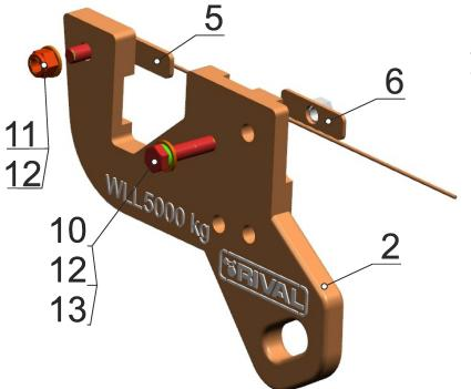
17. Install right recovery point (2) to the chassis, fix it by bolt M12x50 (10) and washers (12) (13) to insert nut (6). Also fix it by nut M12 (11) and washer (12) to insert nut (5).
