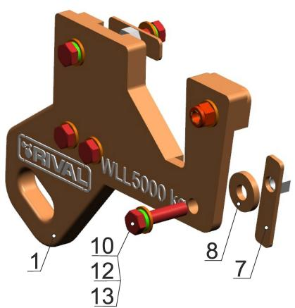
19. Mount recovery point (1) to bracket (3) in same way as in step 18.
