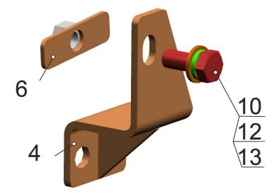
16. Mount brackets (3) (4) to the chassis from inner side and fix them by bolts M12x30 (9) and washers (12) (13) to insert nut (6).
