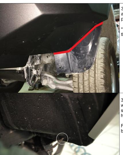
34. Push the flaps to OE plastic fenders and mark the cut line, then cut OE plastic fender.
