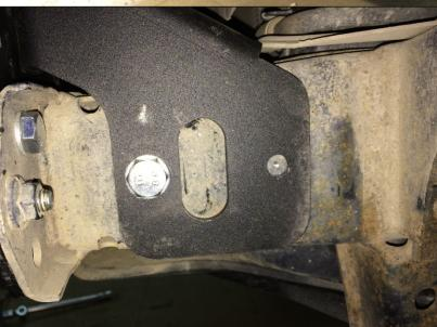
20. Fix adjusting brackets (6, 7). Fix them to winch bracket by bolts M10x25 (14), nuts M10 (22) and washers (25).
