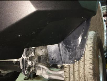
33. Install flaps using bolts M6x20 (18) and washers (24). Make sure the flaps are fixed inside of the bumper, not outside.
