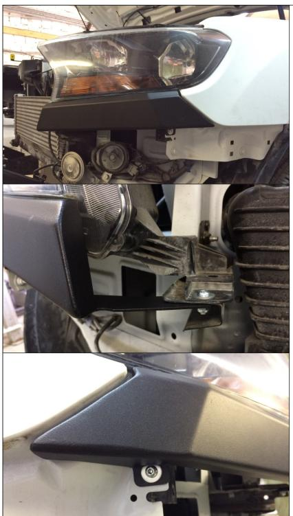
17. Mount under light panels (10 and 11). Fix them with bolts M6x20 (18), nuts M6 (20) and washers (24).
