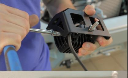
25. \* Mount LED lights into brackets (3). Tighten the joints.
