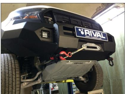
37. Fix underbody armour to the bumper body using OE bolts.
