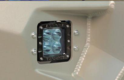
26. \* Install brackets with LED lights onto the bumper using bolts M6x16 (17) and washers (23). Adjust to desired position.
