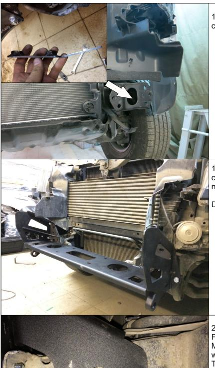
18. Place insert nuts (12) into the chassis.
