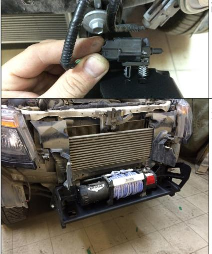
21. Fix temperature sensor to the bracket.
