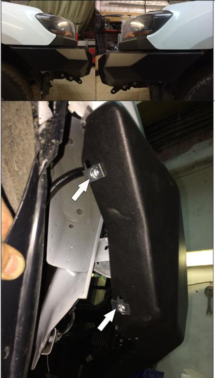
29. Adjust bumper until you have an equal gap between vehicle body and the bumper on both sides. Tighten bolts after that.
