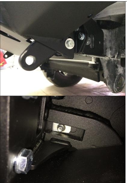
27. Install bumper body (1) onto thewinch bracket (2). Fix its lower part to brackets using bolts M10x30 (15), insert nuts M10 (5) and washers (26).
