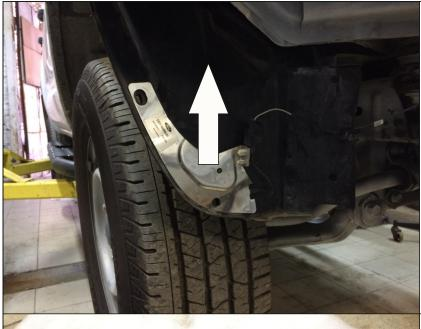
31. From right side, unstick antenna from the fender. Move antenna upper under the bar.
