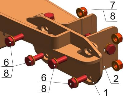
18. Mount winch bracket (1) to the chassis. Fix it to brackets (2, 3, 4) by bolts M10x30 (6), nuts M10 (7) and washers (8).
