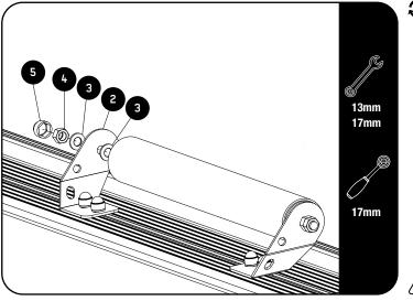
Remove two of the M10 Hex Nuts on the one side of the roller assembly and discard them. "See Note below"
