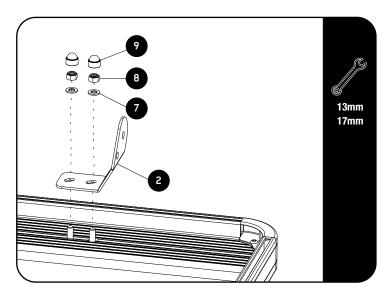
Place the Mounting Brackets (Item 2) onto the Rack, lining up the holes with the Hex Bolts inserted earlier. Loosely secure the Mounting Brackets to the rack using four M8 x 16 x 1SS Flat Washers and four M8 Nyloc nuts supplied (Item 7,8 & 9).
