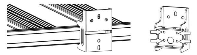
( **B** ) Drill a 6.5 mm hole on each marked positions.
