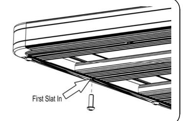
( **D** ) On the chosen side, slide two M8 Nyloc Nuts (Item 5) dome side down into the T-slot channel through the gaps in each corner of the Rack as shown. Slide the two Nyloc Nuts down the channel and line them up with the first Slat in either end.
