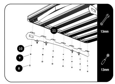
Fit your roof rack to the Foot Rails using M8 x 20 Hex Bolts, M8 x 16 x 1.6SS Flat Washers and M8 Nyloc Nuts (Items 9, 10 & 11).
