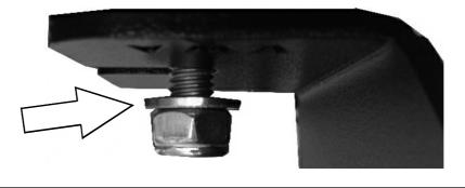
(**C**) Using a tape measure, center the Rack - left to right. Fasten all the Nyloc Nuts securing the Rack to the Foot Rails. To complete the installation, place the M8 Nut Caps (Item 4) supplied over all the Nyloc Nuts.
