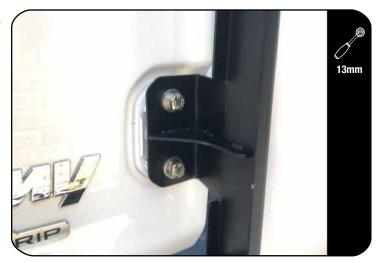
Insert the two 10mm Spacers (Item 8) between the Hinge and the Ladder. Guide the M8x40 Hex Bolt with a M8 Spring Washer and M8 Flat Washer through each mounting slot and spacer and loosely tighten (Item 16, 15 & 14).
