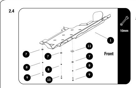
Secure the Front Sump Guard (Item 1) using same mounting points as the factory sump guard. Use two M6 x 25 Hex Bolts, M6 Spring Washers, M6 x 19 x 1SS Flat Washers and 30 x 6 x 2 Washers (Items 7, 8, 9 & 11) on the front of the Sump Guard.
