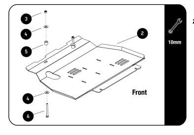
Loosely fit the Rear Sump Guard (Item 2) using M8 x 70 Hex Bolts, M8 x 25 x 2 Flat Washers and M8 Nyloc Nuts (Items 3, 4 & 6).
