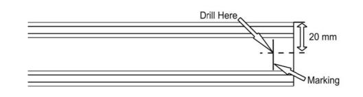
(E) Place the Extrusions back into the vehicle and line them up with your markings from Step 2C. Mark the position of each 8.5mm hole from Step 2D onto the vehicle and remove the Extrusions.
