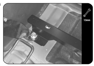
Before securing the mid Cross Member B (Item 3), loosen the rear seat belt bolts.
