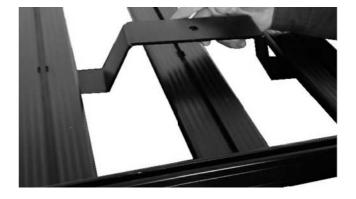
(E) Working from underneath the Rack, line up the Hex Bolts from Step 2B with the machined slots in the Rack as indicated. Lift the Bracket, inserting the Hex Bolts into the machined slots. Slide the Bracket Assembly into position (Left to right) making sure the Hex Bolts remain in the Racks "U" channel.
