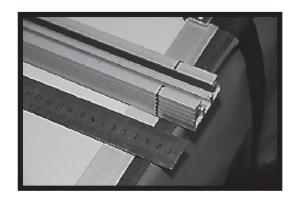
**C)** Cut all 4 ends! Use a hack saw or other tool of choice for cutting through aluminum.
