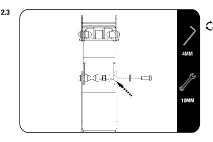
Note the position of the Washer between the upright and Lockable Strap For Water Cap.
