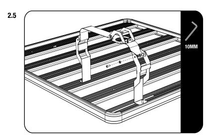
Assemble the Lockable Strap For The Water Cap to the upright brackets by placing it on the inside of the upright brackets. Use the fasteners that you removed in Step 2.2.
