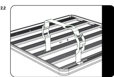
Remove the Nut Caps from all four bolts connecting the Strap to the uprights.
