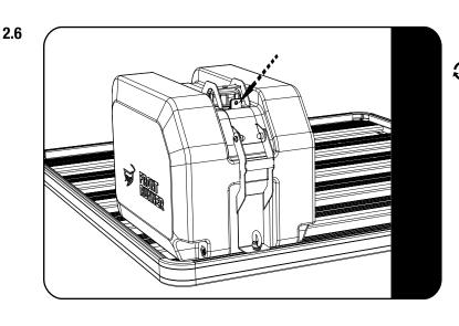
Place the Water Tank into position and close the Strap. Refit the Eye-Nut that secures the tank.
