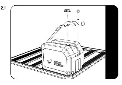
Loosen and remove the tank cap and the Eye-Nut that holds the tank in place and then remove the tank from the Rack.
