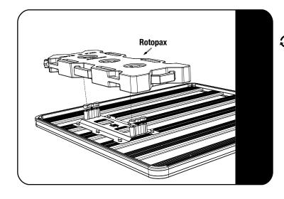
Place the Rotopax over the RotoPax RX-PM Pack mounts and tighten.
