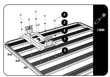
Slide 2 M8x16 hex bolts (item 5) into each of the 2nd, 3rd and 4th slats t-slot. Place the Rotopax mounting plate (item 1) over the bolts. Move the mounting plate into the desired position by using the Rotopax tank before securing it with items 3 and 4. Finnish it of by placing a M8 nut cap (item 2) over each of the 6 nyloc nuts (item 3).
