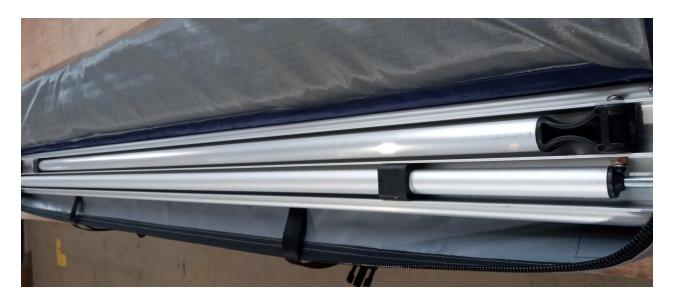
Once attached to the vehicle securely, there are two extendable aluminium poles in the awning base attached to the vehicle, these swivel out horizontally at 90 degrees to the vehicle and connect to the secondary extruded aluminium section at the outer end of the awning. In the secondary outer section are two more extendable aluminium poles, both of which swivel out 90 degrees vertically to the ground. These two poles are each restrained by the guy ropes and ground pegs provided.
