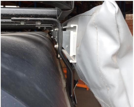
Once attached to the vehicle securely, there are two extendable aluminium poles in the awning base attached to the vehicle, these swivel out horizontally at 90 degrees to the vehicle and connect to the secondary extruded aluminium section at the outer end of the awning. In the secondary outer section are two more extendable aluminium poles, both of which swivel out 90 degrees vertically to the ground. These two poles are each restrained by the guy ropes and ground pegs provided.
