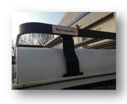
Only when you are happy with the position tighten the gutter clamps evenly taking care not to over tighten. Finally tighten all the leg mounting bolts.
