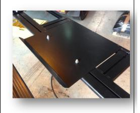
2. Using the access slots slide the leg mounting bolts into position.
