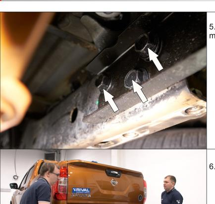
5. Unscrew 3 bolts of rear bumper mount from left and right side.
