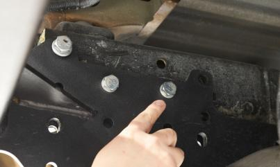
14. Mount bracket (2) from left side of vehicle into OE hole using bolt M12x1,25x40(12) and washer M12x24(17). Do not tighten yet.
