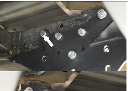
13. Mount bracket (2) on inside nut M10 (5) using bolt M10x40 (10) and washer M10x20 (16). Do not tighten yet.
