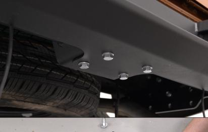
22. \*Mount bumper body (1) on bracket (2) in lower part using bolts M12x40(11) and washers M12x24(17). Tighten all screws.
