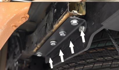
17. Mount bracket on reinforcement using bolts M10x40 and washers M10x20. Do not tighten yet.
