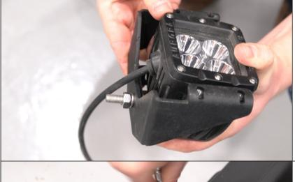
18. \*Mount lights (19) on brackets (4) using fittings from light set. \*For package with LED lights.
