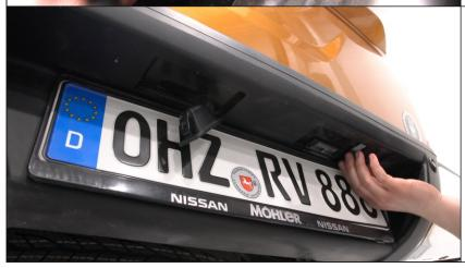
4. Remove license plate lights. Gently pull lights down, turn wire and light for a 90 degrees.
