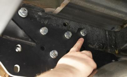
15. Mount inside nut M10(5) into the vehicle frame from the left side.
