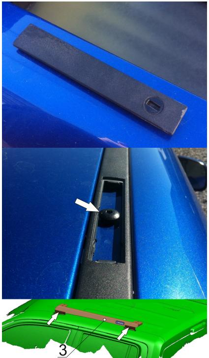
1. Remove plastic lockers on the roof of the vehicle.
