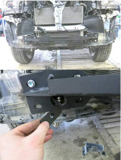
11. Install winch bracket (1) to the chassis using factory bolts, bolts M10x30 (6), nuts M10 (10) and washers (14).
